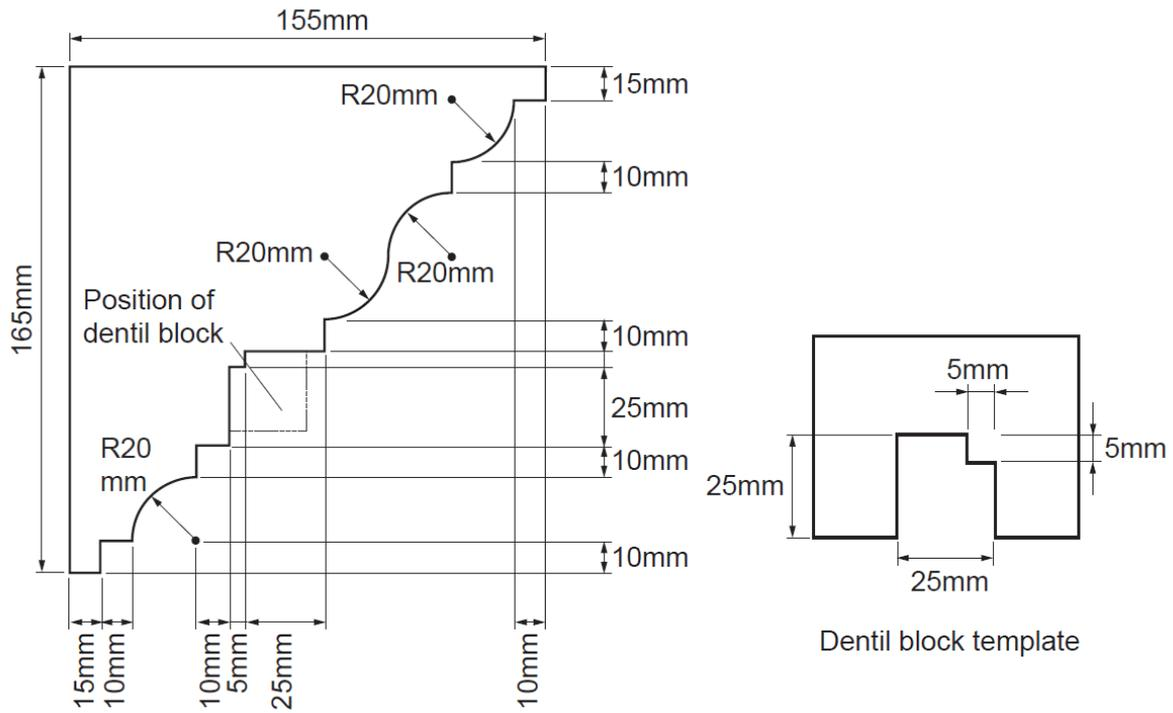
**Figure 2 – Double slipper running mould**
