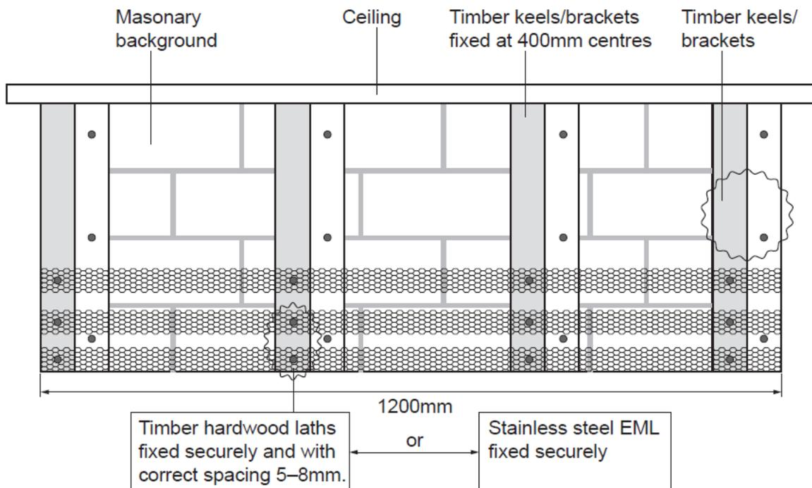
**Figure 2** – Section through completed work/completed drawing
