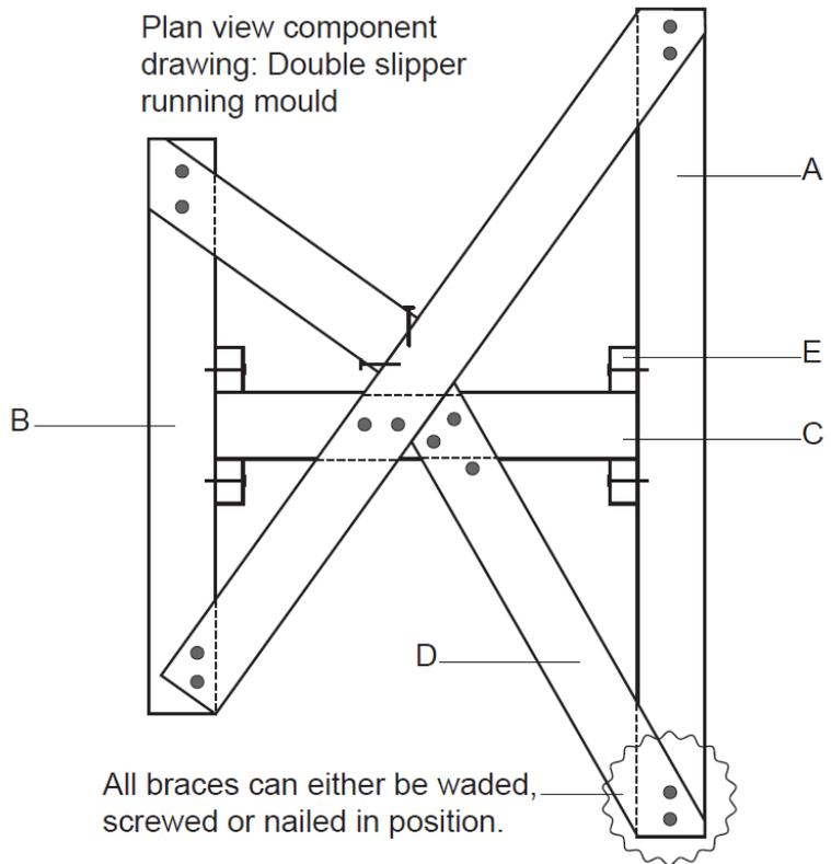
**Figure 3** – Component drawing of model
