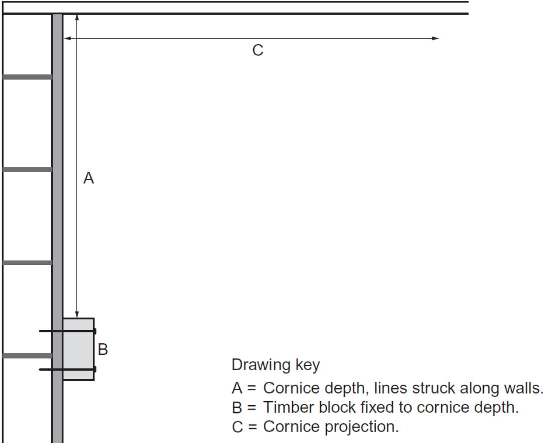
**Figure 3 – Fixing and finishing the cornice**
