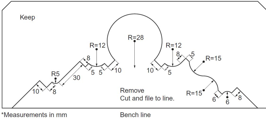
**Figure 2 – Stock of running mould**
