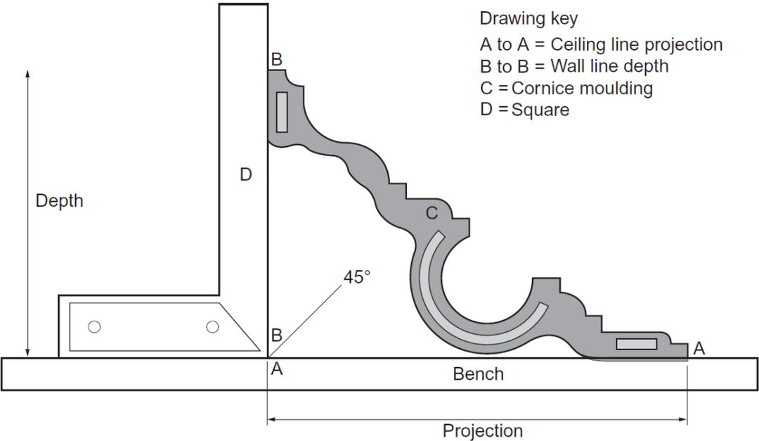
**Figure 2** – Setting out to fix the cornice
