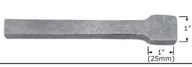
Take a short **yellow** heat up to the mark. If necessary, quench to just short of the mark.
