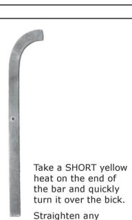
Straighten any distortion in the rest of the bar.
