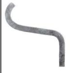
Take a short yellow heat on the end. Quickly bend the end over the tip of the bick, being careful not to reduce the width.
