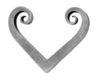
Scroll the two ends using hammer only.
