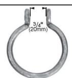
Take a heat on about a quarter of the length, quench the eye to prevent distortion and bend over the bick. Repeat on the other end.
