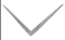
Starting almost in the corner, draw out each arm to an even taper of equal lengths.
