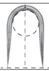
Take an even heat on the middle section and bend around until the legs are parallel.
