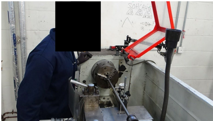
Candidate proving that tailstock was realigned using DTI
