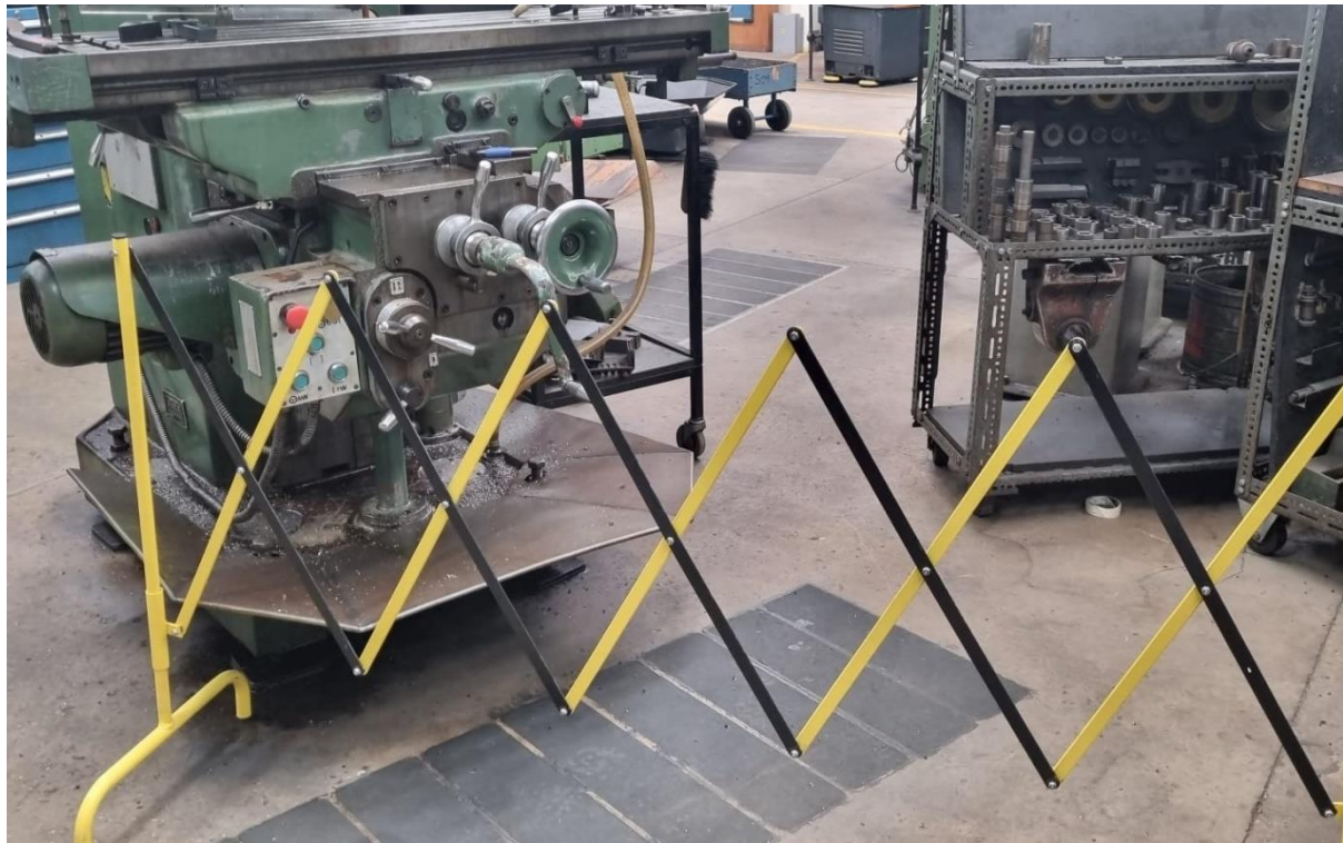
Photograph 6: Photographic evidence showing the wider working area after subassemblies removed from the milling machine, with parts, components and sub-assemblies placed in separate containers not in view, with a clear floor and safety barrier in place. Clean and tidy working area with spare parts organised and on hand.
