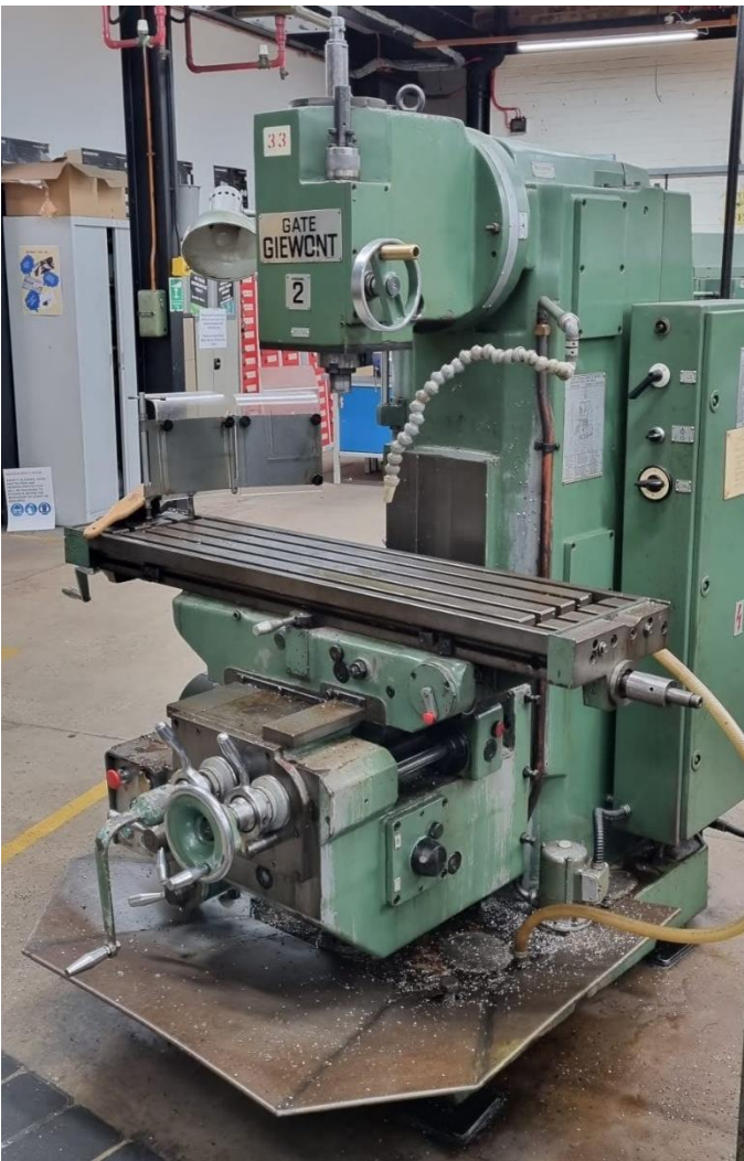
Photograph 2: Photographic evidence showing the condition of the full milling machine prior to any work being carried out. The candidate noted the debris and burr around the base of the machine from being previously used.
