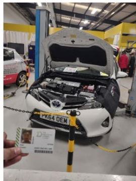
Prepared work area with VPE.
