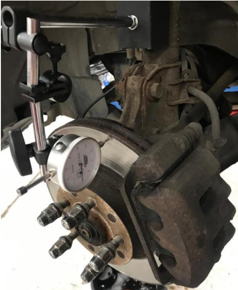
Photograph 4: Photographic evidence shows the set up and accurately positioned DTI gauge to take brake run out readings, arm connected to the suspension correctly and gauge fitted to take accurate readings.
