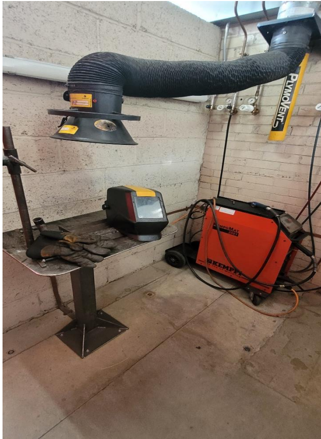
Photograph 1: Photographic evidence showing the prepared welding area, using heat proof gloves instead of long-sleeved welding gauntlets.
