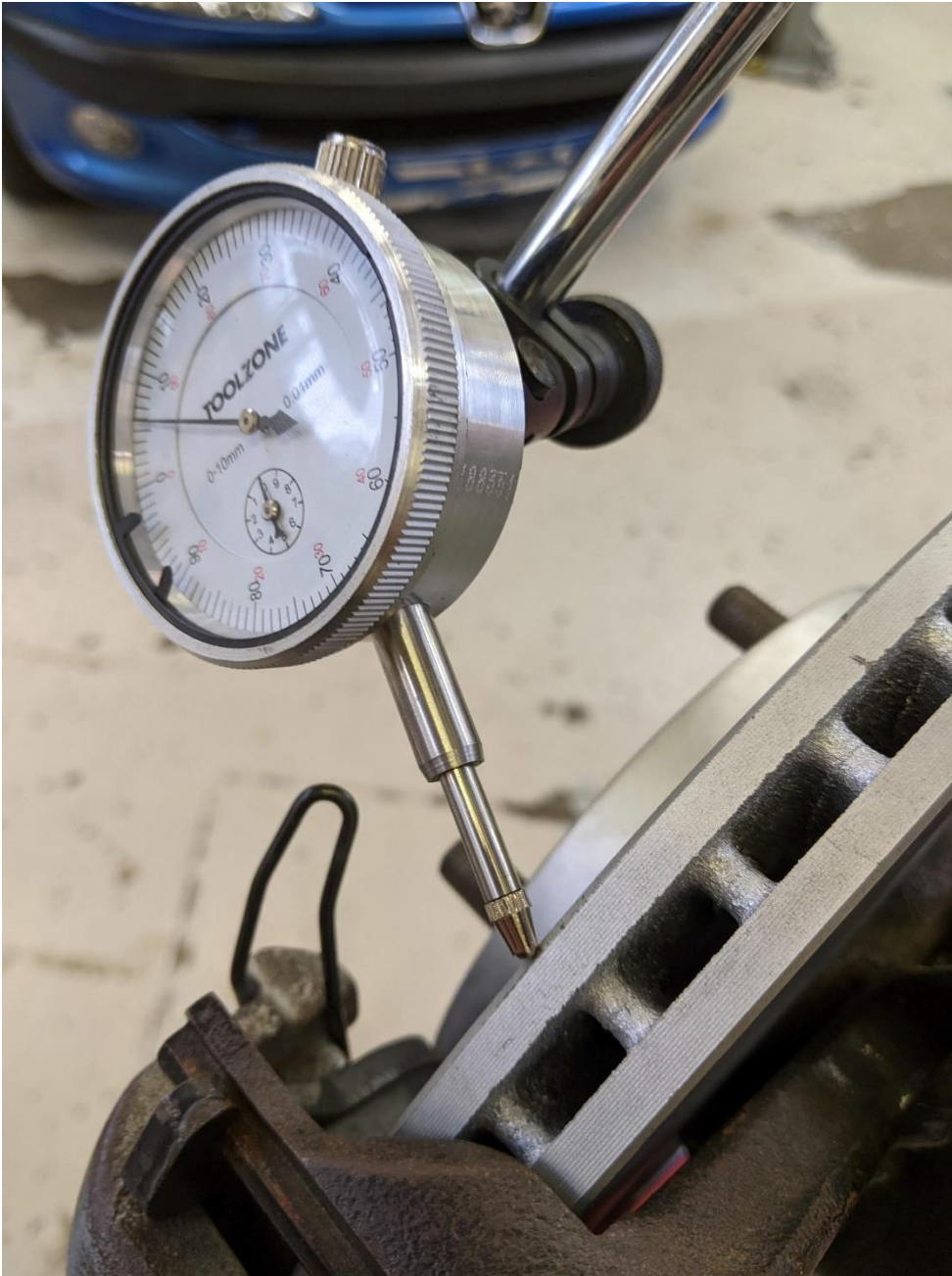
Photograph 3: Photographic evidence shows the initial set up and positioned DTI gauge to take brake run out readings, gauge has been set up to touch the outer edge of the disc which will give an inaccurate reading. This was subsequently corrected when the candidate realised the mistake and realigned.
