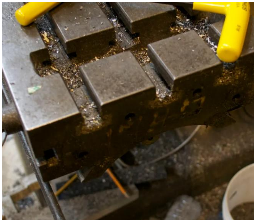
Photograph 6: Power feed removed showing burr has not been cleaned away and tool lying on top.
