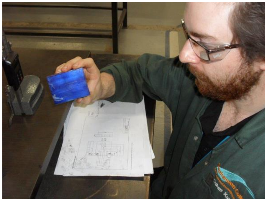
Photograph 7 - showing the preparation of the material, the application of engineer's blue to stock. This should be an even application and no excess or spillages.
