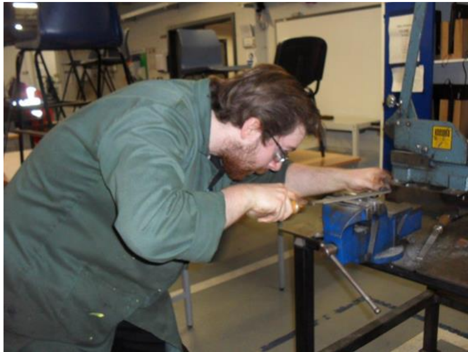
Photograph 7 - showing the preparation of the material, the application of engineer's blue to stock. This should be an even application and no excess or spillages.
