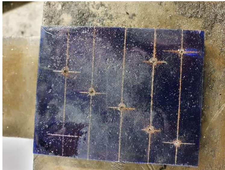
Photograph 11 – showing an example of where a threshold competence level candidate has incorrectly set out the hole pattern resulting in some misalignment of the holes on the finished component.
