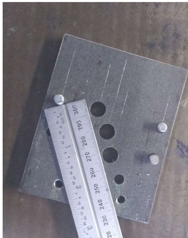
Photograph 11 – showing an example of where a threshold competence level candidate has incorrectly set out the hole pattern resulting in some misalignment of the holes on the finished component.
