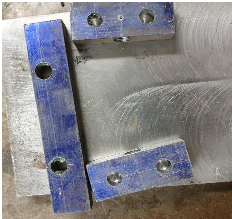
Photograph 8 – showing the front support block and the two side supports components, prior to finishing.
