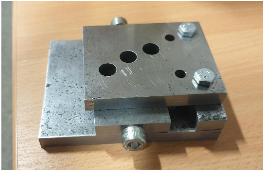
Photograph 10 – showing the completed drill jig assembly. The alignment of the parts is good. The surface finish meets the drawing requirements, all millscale has been removed to a true surface finish. All parts are flush and in line. The side supports are interchangeable and can be used on either side. The dowel pins (not shown) are flush with the base plate.
