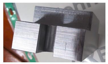
Limited marks, however there are very faint 4 jaw marks, despite using shim to protect his work.
