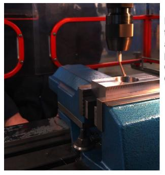
Datuming the centre of the die block, this then allowed all the other processes to be calculated from the centre.
