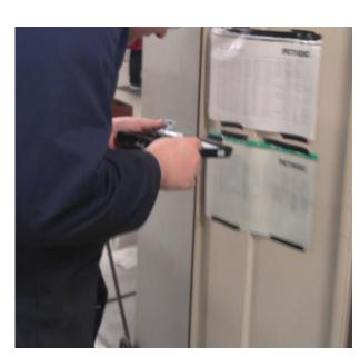
equipment was checked out against the serviceability record. also did visual checks on the equipment for example checking the depth mic was reading 0 by checking it on the surface table.
