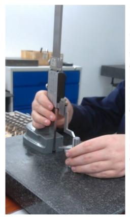
Many different measuring techniques used to do the final checks. Here has placed the correct size slip gauges in the U'cut and then used the digital height gauge to measure the length of the thread in the CNC part.
