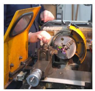
All lathe tools were check to find if they were on centre height before starting the turning operations. Particular when the 4 jaw chuck was being used as this couldn't hold the centre finder to assist with the height of the tool. This was forward planning.
