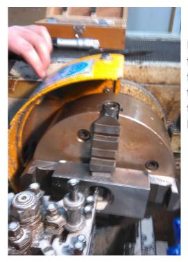
Using the final finishing boring tool to bore out the final sizes of the bore in the die block.
