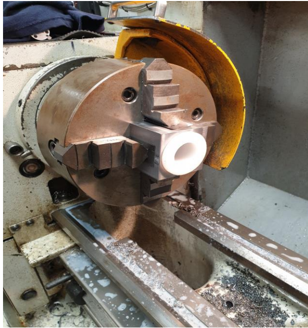
Photograph 9 – showing the bored out bearing housing, some additional adjustment was required until the nylon top hat was a push fit.
