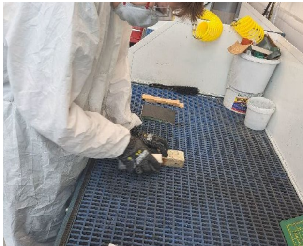
Figure 33 - Trimming using permagrit block
