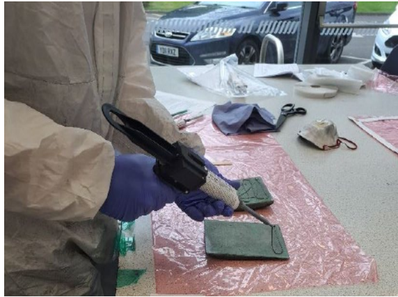
Figure 35 - Application of adhesive
