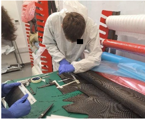
Figure 14 - Cutting dry fibres
