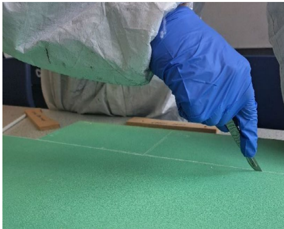
Figure 9 - Cutting of foam
