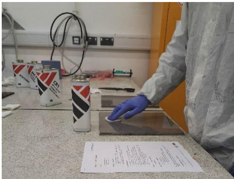
Figure 5 - Application of release agent
