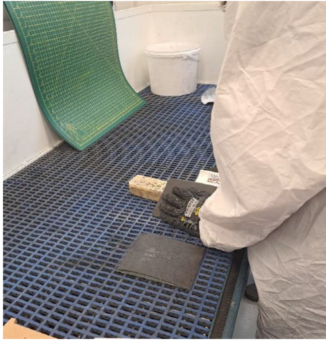
Figure 34 - Trimming using permagrit block
