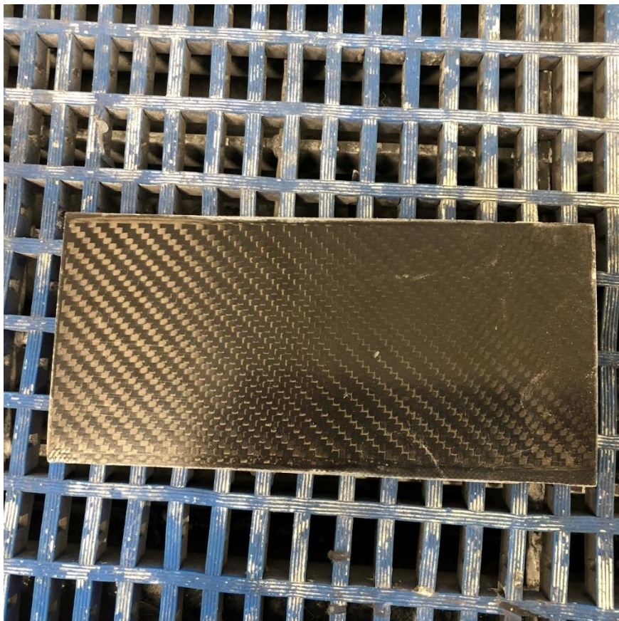
Photograph 42 – showing the final assembly which has been safe edged and ready for machining to final dimensions.
