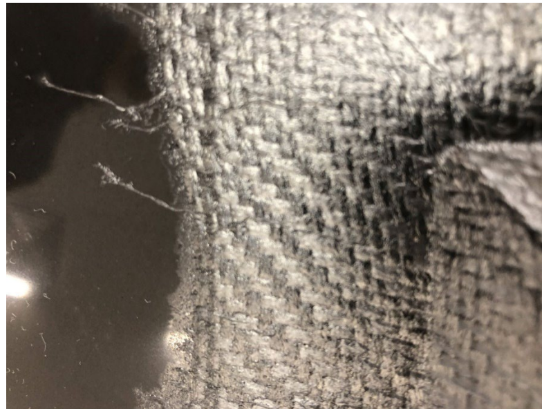
Photograph 24 – showing detail of edges, corners and transitions showing inconsistent definition and orientation of fibre.
