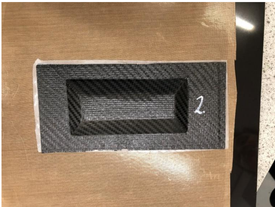
Photograph 34 – showing the spacer block component placed on top of release film. Note bottom left corner has no adhesive film overlap. The film should melt into this area during curing, but it is not good practice. Bottom edge showing some signs of inconsistent trimming activities.
