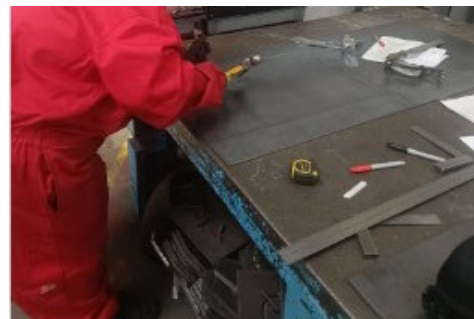
Marking out the metal to be able to cut the metal pieces
