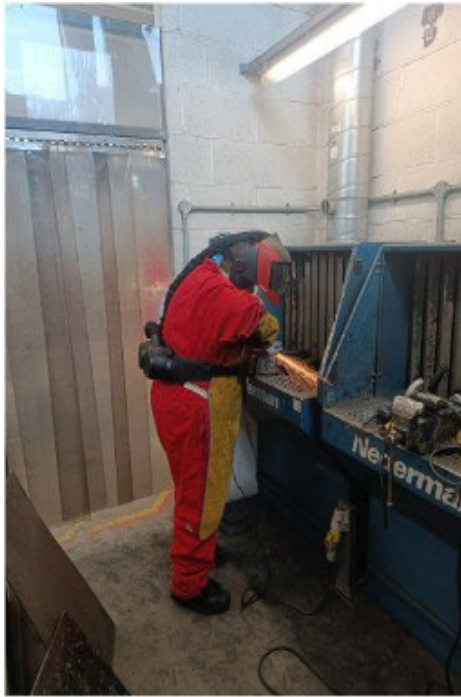
Using grinder for edges of frame box section
