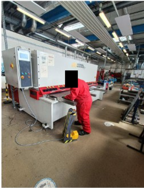
Using the guillotine Making sure that fingers are away from the shield
