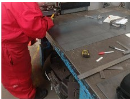
Marking out the metal to be able to cut the metal pieces
