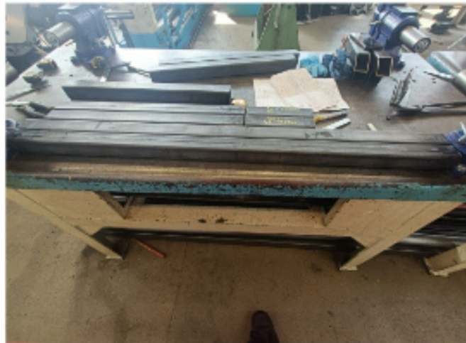
The cut out box section for the frame
