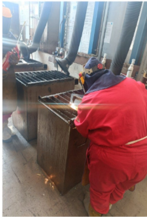
Using oxy-fuel cutting for the plates
