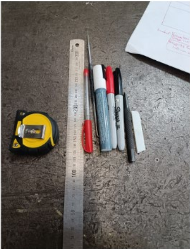
Equipment used for marking out
