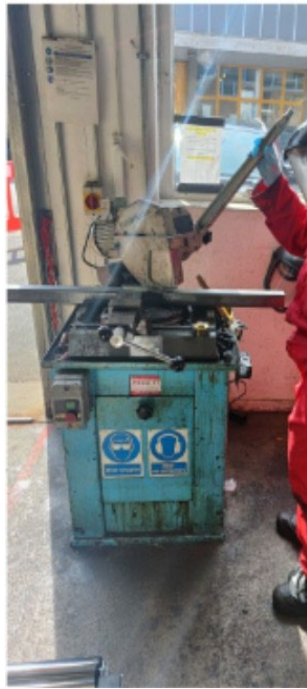
Using the chop saw for the metal frame
