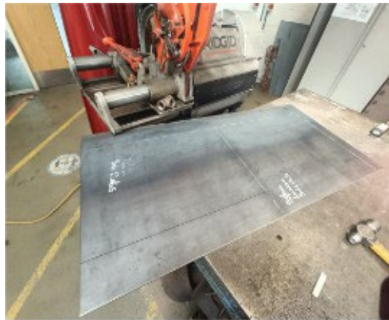
Metal all marked up to use Oxy-fuel Cutting
