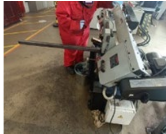
Using the Horizontal Bandsaw making sure that the box section is the right length
