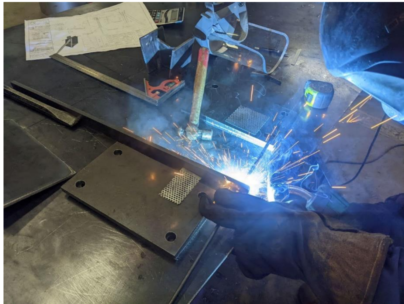
Photograph 14 - showing the welding application, workpiece is secured on the welding table. Full protective equipment is worn.
