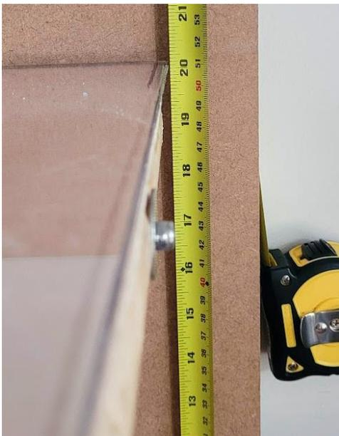
**Photographs 9 and 10** show the platform lift fully extended to the maximum height. In the photograph, the platform is raised to slightly above 500 mm, but it was then lowered to 500 mm, as per the height requirement, using the threaded bar mechanism. The runner rails are neatly cut and are fully functional.
