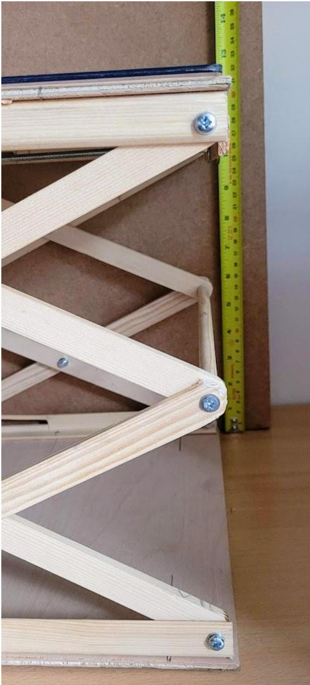
**Photographs 8** shows the platform lift at the halfway point. The lift is functional and can be raised and lowered smoothly as planned using the threaded bar mechanism.
