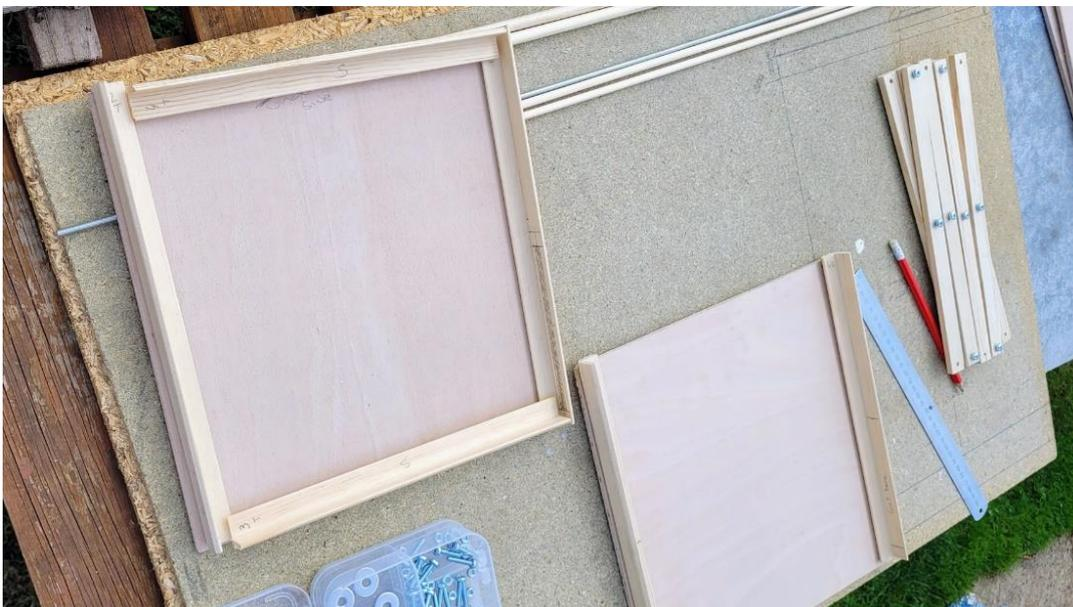
**Photographs 2 and 3** show the sides for the runner rails marked up. The position of the holes for the runners is clearly marked and detailed annotations are included. The candidate has temporarily placed the mechanism sliders in situ for consideration.
