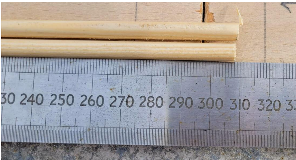
Photographs 4 and 5 show the marking out and the cut pieces. The marking is not very accurate and this resulted in the cutting being 1-2 mm short of the required length of 310 mm.
