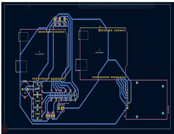
This is the PCB design for the circuit with the recent changes which includes the new RFID and the second Arduino. As you can see on the photo the design looks more complex because there is another Arduino and the RFID wiring which could also mean that it makes longer to make and solder and would also make it a little more expensive because it would require more copper because the circuit itself is bigger.
