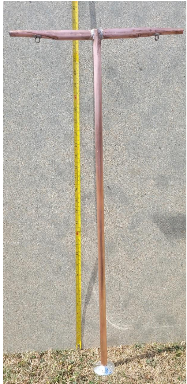
Photographs 6 and 7 show the completed soldered joins of the prototype, demonstrating the taper of the arms. The candidate is using a tape measure to show the accuracy of the length.
