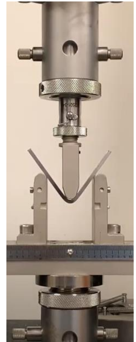
Photographs show the process used for the three point bending test on bar. The left image has the test piece in place, the middle image shows force being applied to the test piece and the right image shows the stress point has been met and the material has folded.
