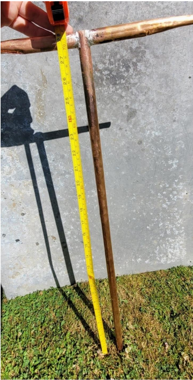
Photographs 6 and 7 show the completed soldered joins of the prototype, demonstrating the taper of the arms. The candidate is using a tape measure to show the accuracy of the length.
