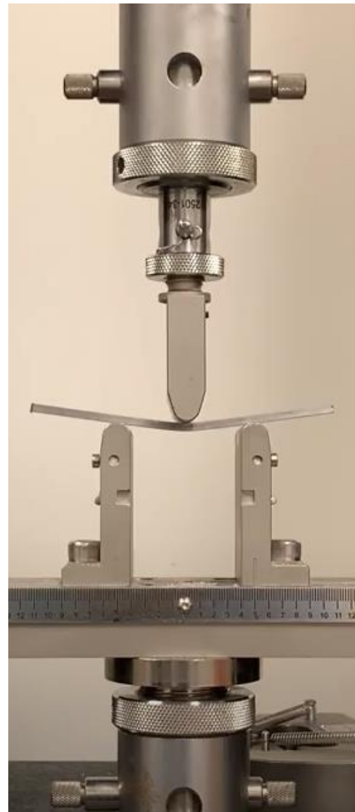
Photographs show the process used for the three point bending test on bar. The left image has the test piece in place, the middle image shows force being applied to the test piece and the right image shows the stress point has been met and the material has folded.
