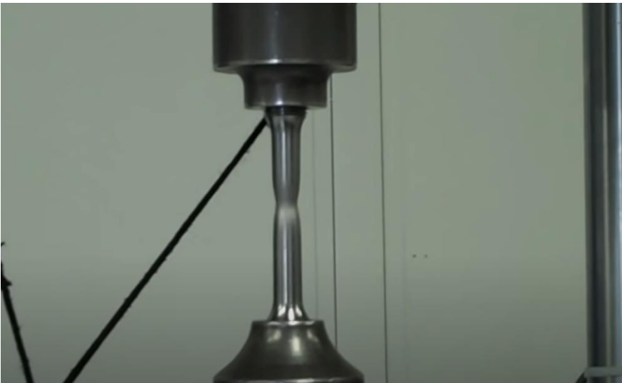
Test piece 'necking' under load.
