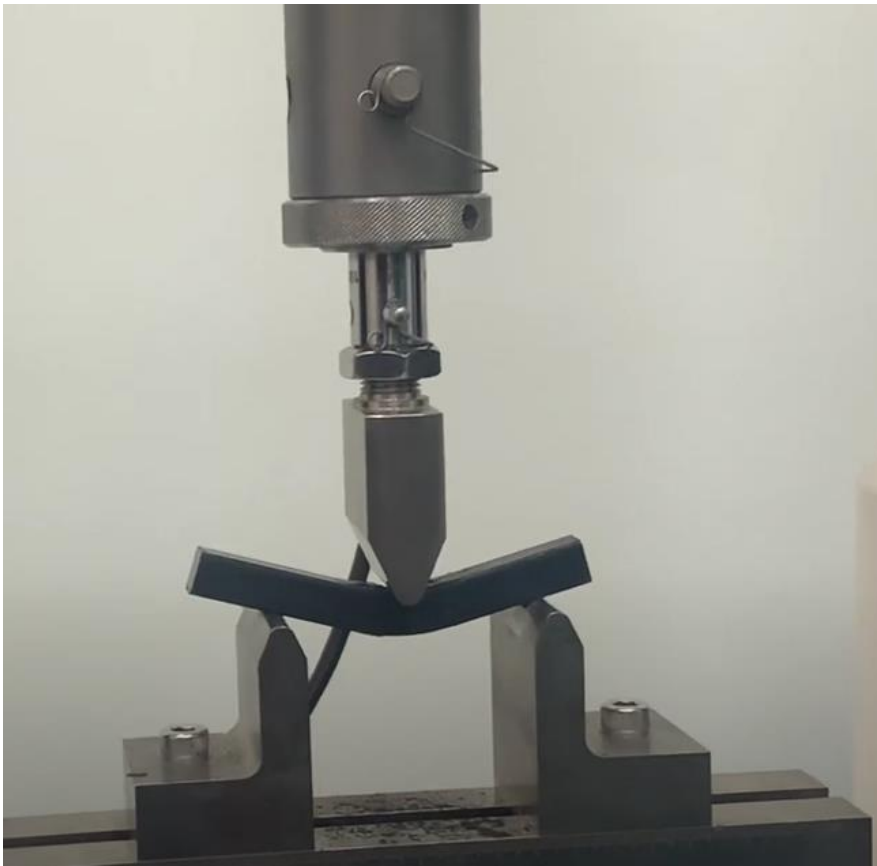
Test piece beginning to show the bend from load applied.
