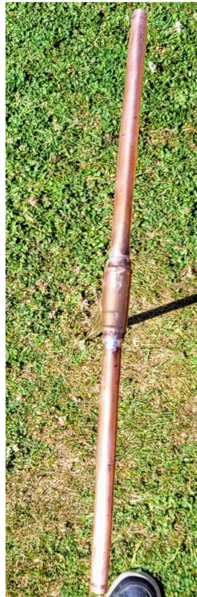
Photograph 9 shows a bird's eye view of the pylon. The join of the arms to the mast from the top is different to the CAD model, as it is soldered flush.
