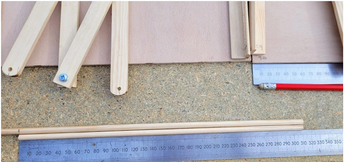
Photograph 6 shows accurate cutting length and measuring to 300 mm, with an extra 10 mm to allow for the prototype to have some fore and aft movement on the runner.
