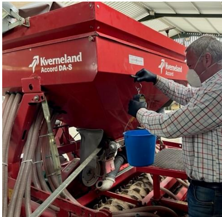
Photo 6 (assessor) Calibration: weighing seed
