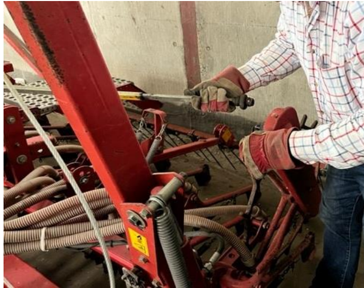
Photo 3 (assessor) Pre-use checks: land wheel drive shaft
