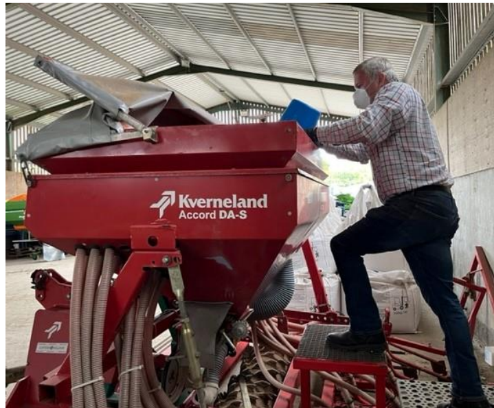
Photo 7 (assessor) Calibration: putting seed back into hopper
