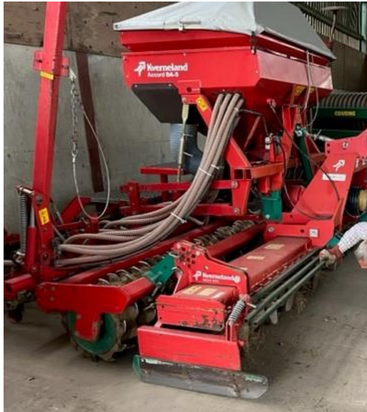
Photo 1 (assessor) Pre-use checks: power harrow tines and carriers
