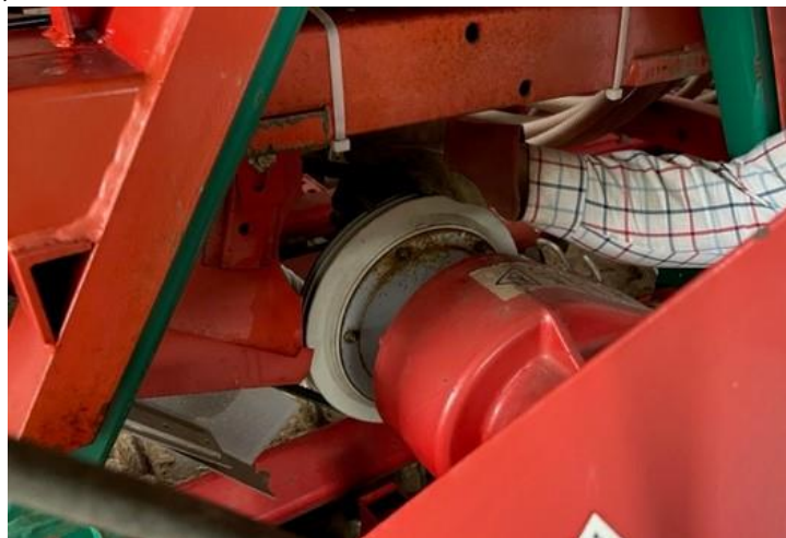
Photo 4 (assessor) Pre-use checks: fan belts
