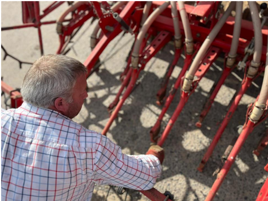
Photo 16 (assessor) Post use checks: inspecting coulters and coulters pipes
