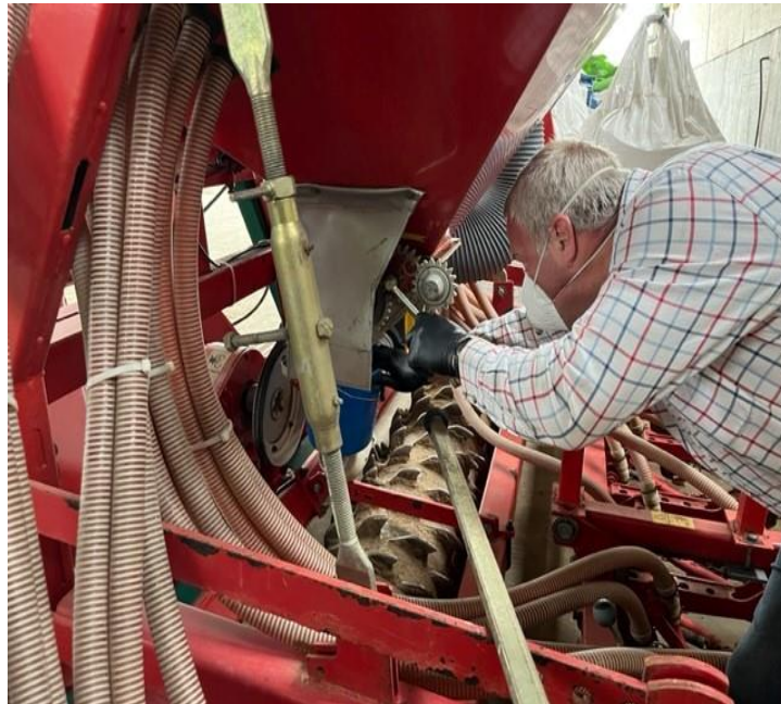
Photo 5 (assessor) Calibration: turning calibration handle
