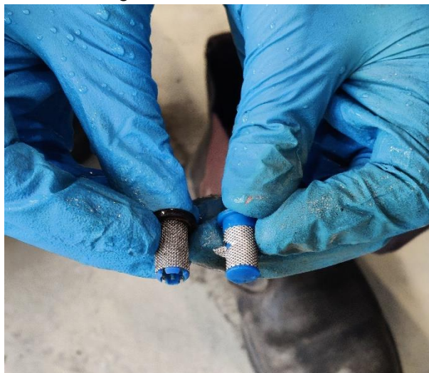
Photo 5 Possible nozzle filter damage
