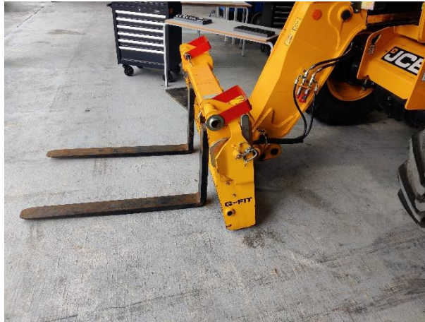
Photo 3 Preparation and immobilisation of the machinery: tines in neutral position
