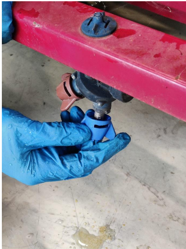
Photo 3 Serviced parts: removed nozzles
