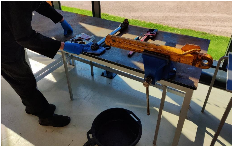
Photo 1 Stripped cylinder before repair
