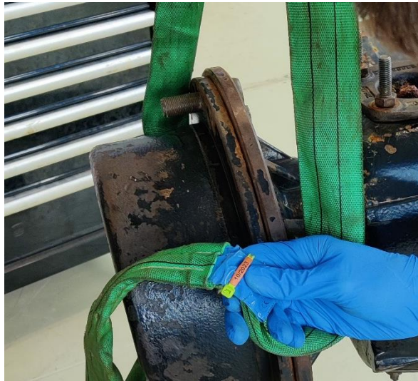
Photo 1 Checking safety of lifting equipment
