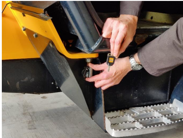
Photo 1 Preparation and immobilisation of the machinery: the machinery once prepared and immobilised: removal of the ignition key
