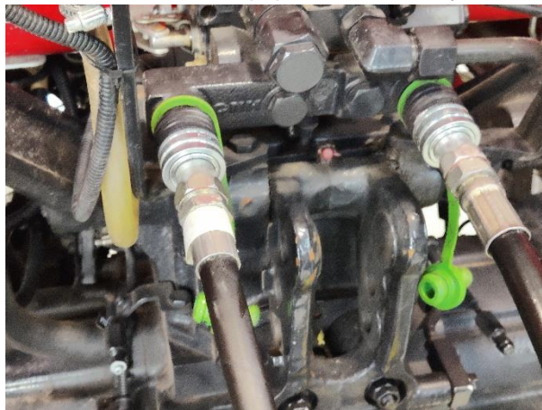
Photo 2 Connecting the tractor to the test equipment: correctly connected
