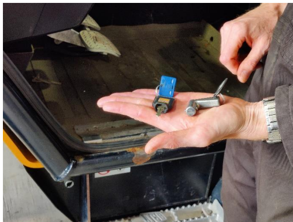
Photo 2 Preparation and immobilisation of the machinery: the machinery once prepared and immobilised: removal of the isolator
