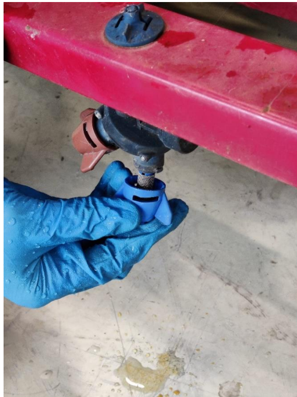
Photo 4 Serviced parts: removed nozzles
