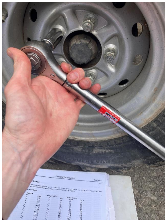
Photo 1 Using the torque wrench: hand, wrench, wheel, and manufacturer’s specification
