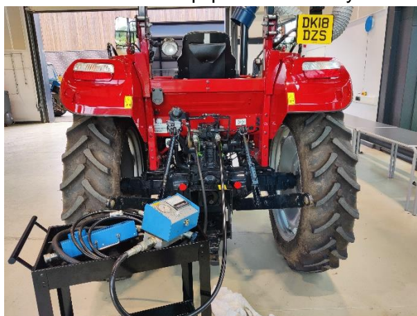
Photo 3 Connecting the tractor to the test equipment: correctly connected
