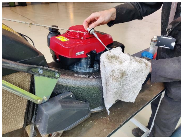
Photo 2 Lubrication level of mower
