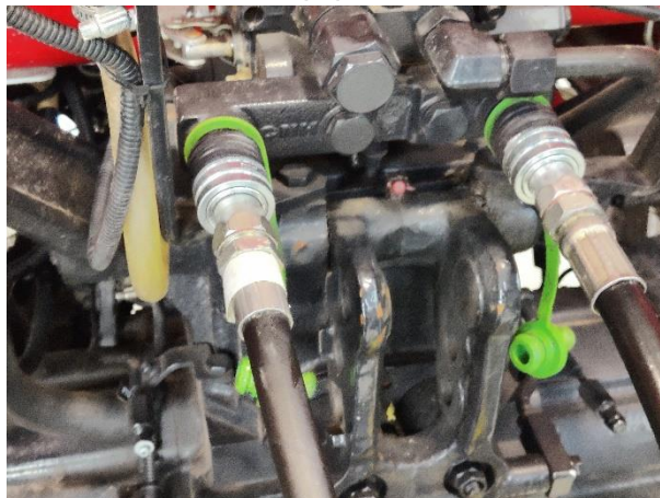
Photo 2 Connecting the tractor to the test equipment: correct connection (second attempt)
