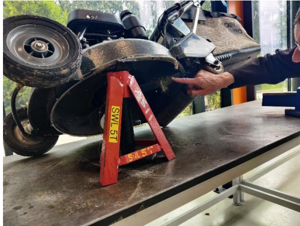
Photo 1 Mower supported for safe working
