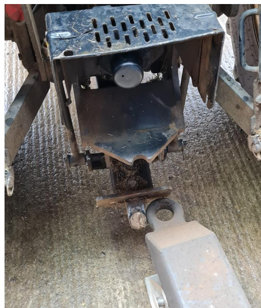
4. Pick up hook is off centre to the left of the trailer ring
