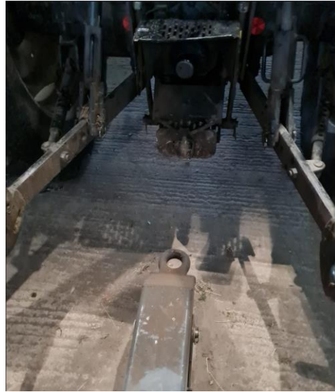
2. Tractor correctly aligned to trailer
