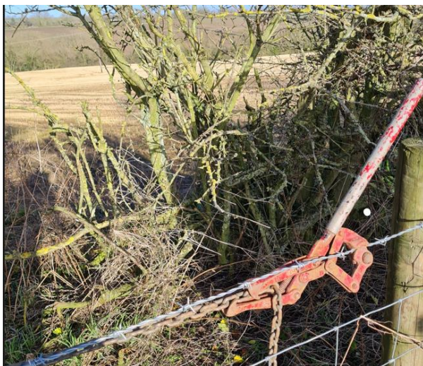
The strainer in place
