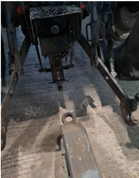
3. the hook lowered to just above the ground in preparation to go under the trailer drawbar ring
